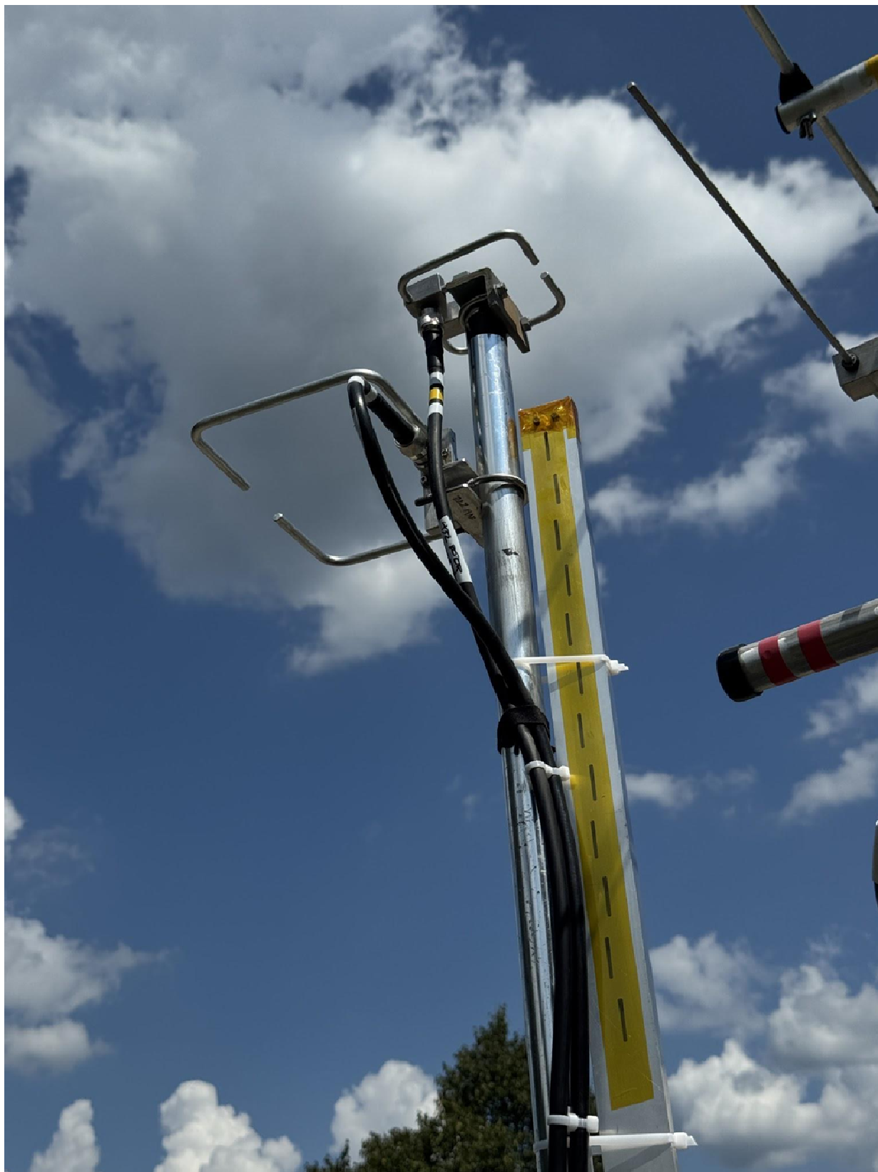
5 GHz Slot Antenna with 12 Slots (2) Bays fabricated by PE1RKI for the 222 and Up Contest
