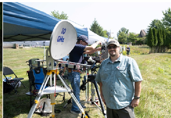
Andy WA4BRX with his Offset dish, with dual 10 & 24 GHz feed. KC6QHP photo
