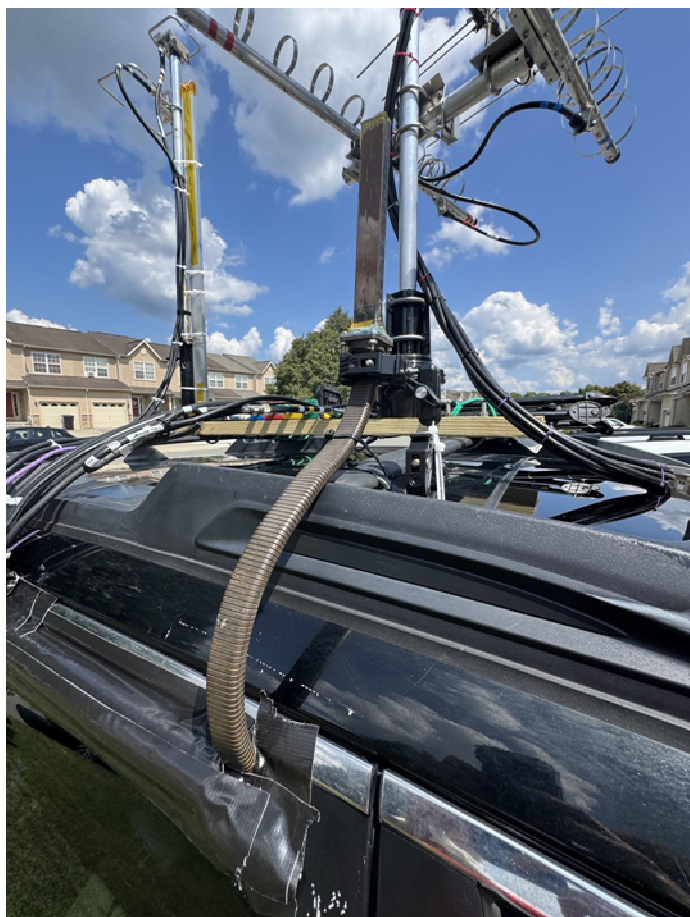
Universal Super Clamp for Motorcycles to temporarily mount the Slot Antenna with flexible Wave Guide
