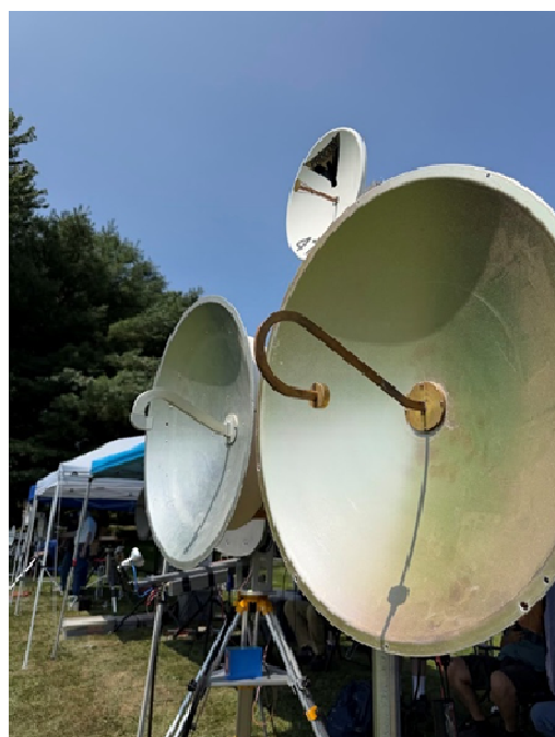
Dave K1RZ's 10, 24 & 47 GHz Dish Antenna's. KC6QHP photo
